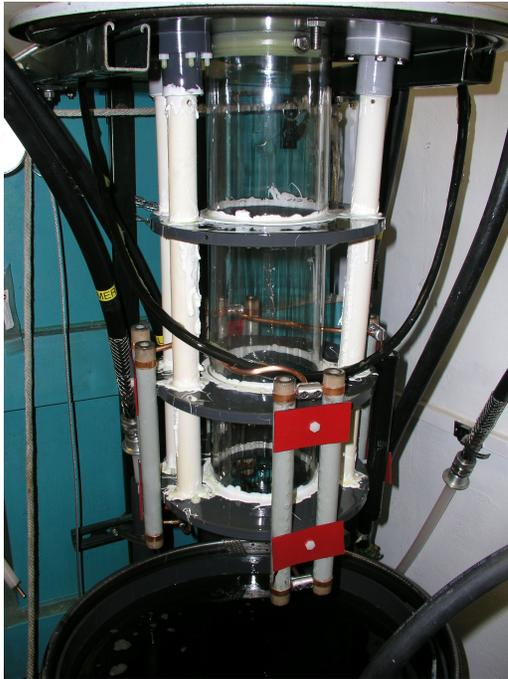
Present Resistor Barrel → No arcs in IEC device during the test
