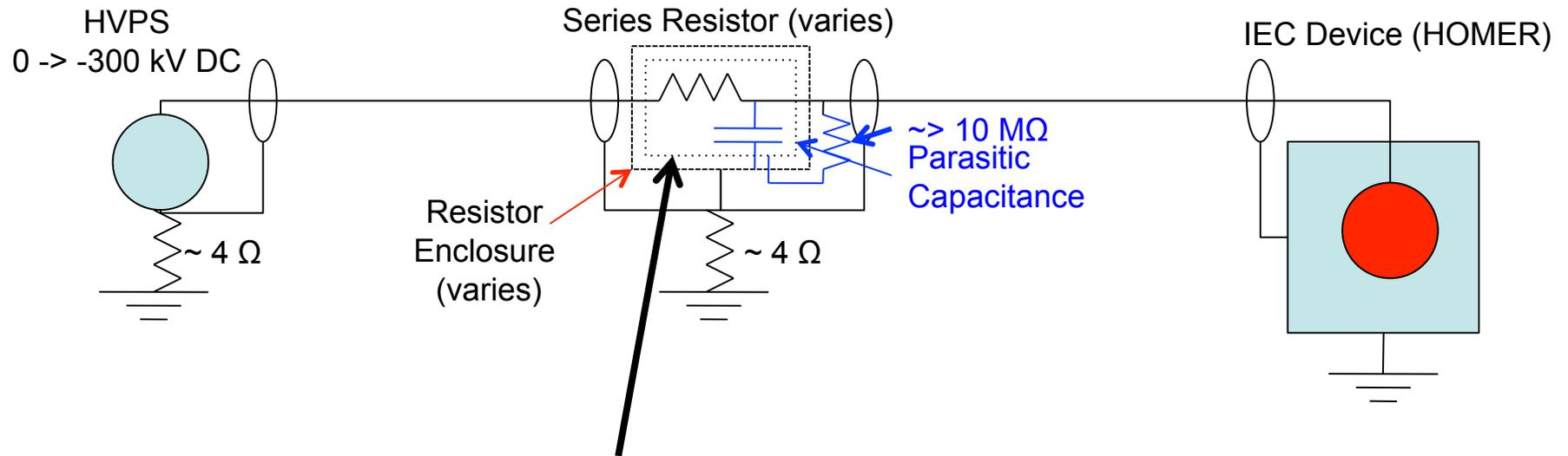
A driven guard shield, properly designed, should greatly reduce the parasitic capacitance that exists between the series resistor assembly and the enclosure.
