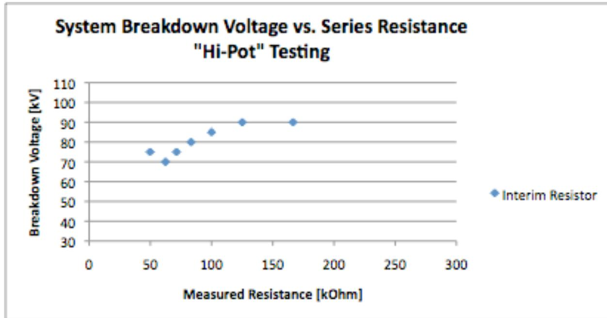
The system with the interim resistor assembly is not stable either!
