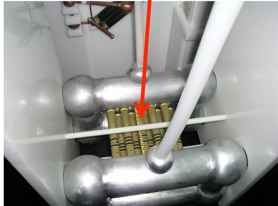
The interim resistor array, like the switch, passed “hi-pot” tests to 100 kV in air when **NOT** connected to an IEC device.
