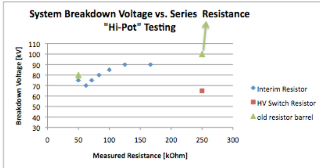
*If the old resistor barrel is modified to have only 50 k $\Omega$  resistance, then the system is also unstable*
