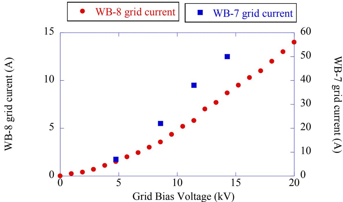
For the same grid bias: WB-8 operate with lower grid current than WB-7, while WB-8 has 6x higher plasma density (WB-8:  $3 \times 10^{12} \text{ cm}^{-3}$  and WB-7:  $5 \times 10^{11} \text{ cm}^{-3}$ )
