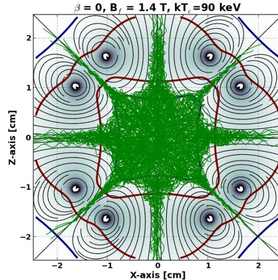
Low  $\beta$  cusp confinement can be modeled as “magnetic mirror” with particle transit time as a scattering time to loss cone: due to non-conserved magnetic moment near  $r=0$
