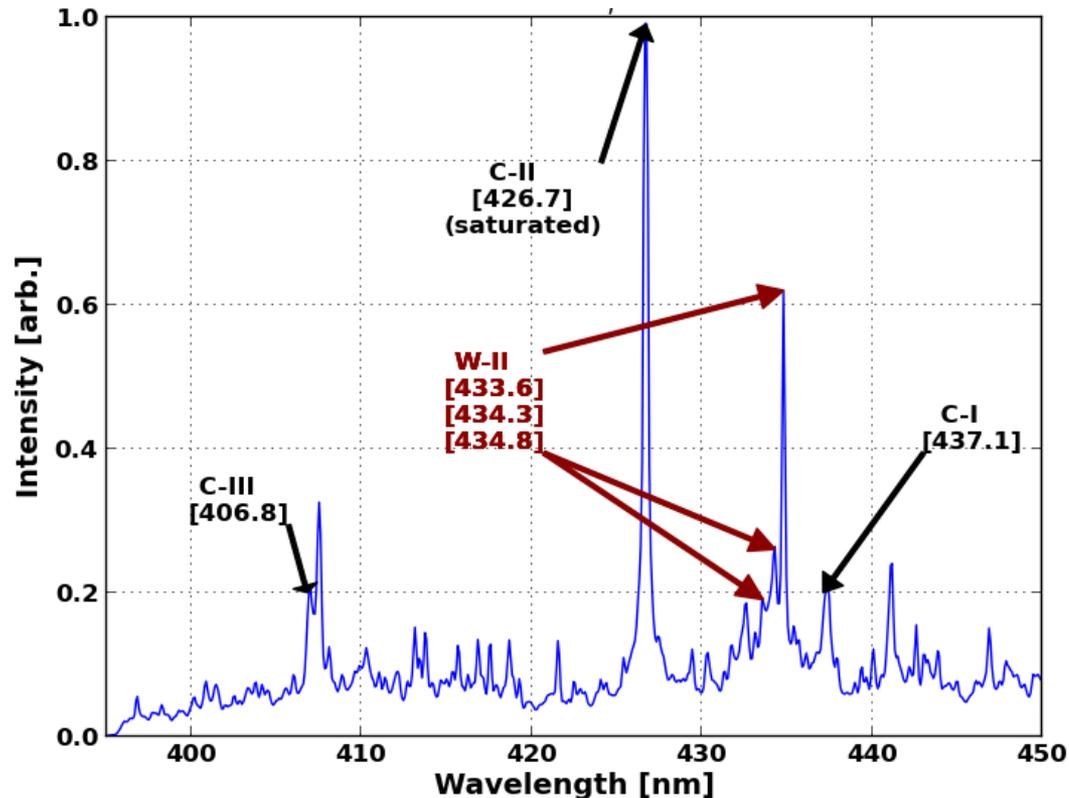
**During the high  $\beta$  phase, plasma emission shows strong C<sup>+</sup> lines & presence of W<sup>+</sup> lines**
