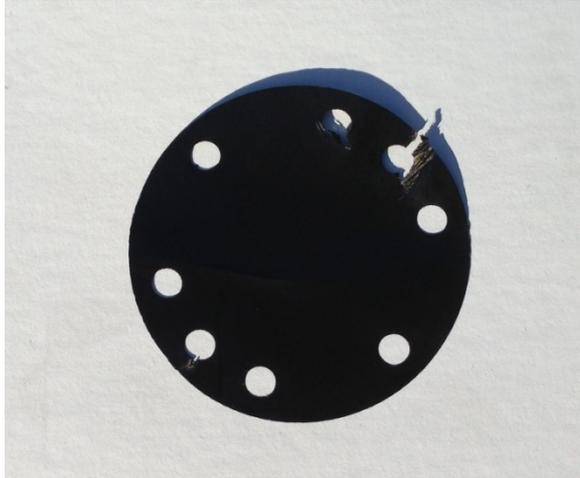
25  $\mu\text{m}$  thick light tight Kapton filter
