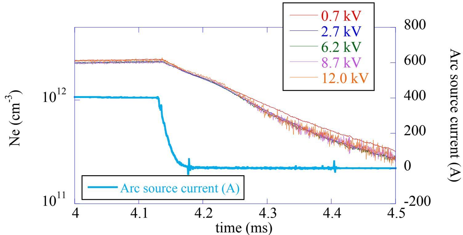
*No change in  $n_e$  decay time ( $\sim 180 \mu\text{s}$ ) vs. grid bias voltage*
