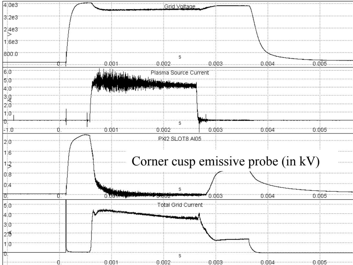
Plasma potential at the corner cusp drops to 0V with increasing plasma density
