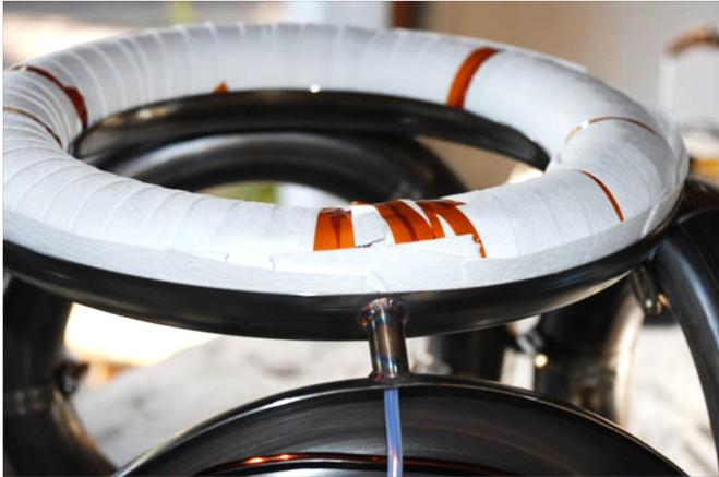
6 coil system with joints
