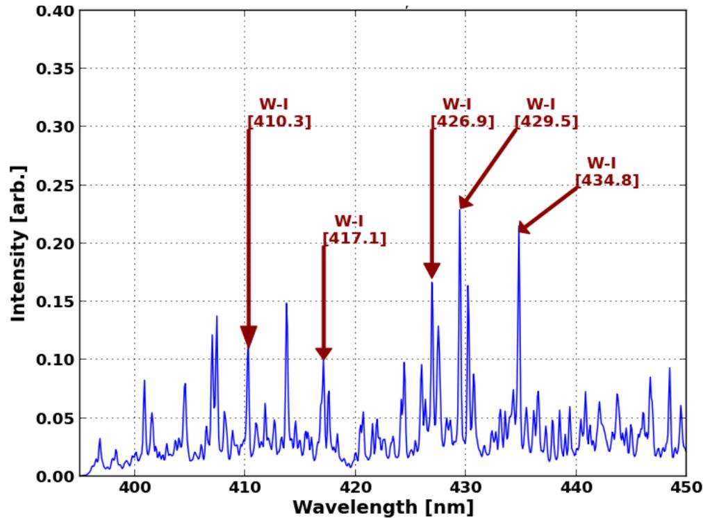
At later time, plasma emission is dominated by W neutral lines, while  $\text{C}^+$  and  $\text{W}^+$  lines disappear
