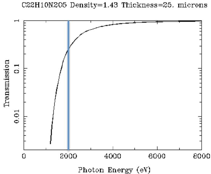
Filter has sharp cutoff at  $\sim 2$  keV photon energy
