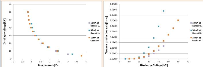
Fig.8. Discharge characteristic with D<sub>2</sub> gas
