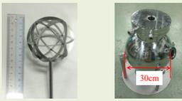
Fig.4. Cathode Fig.5. Vacuum chamber
