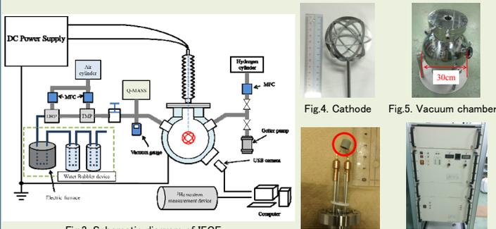
Fig.3. Schematic diagram of IECF
