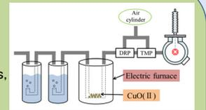
Fig.15. Schematic diagram of Water Bubbling Recovery
