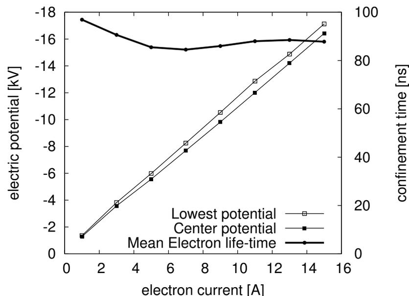
(b) Well depth and confinement time as function of total e-gun current.
