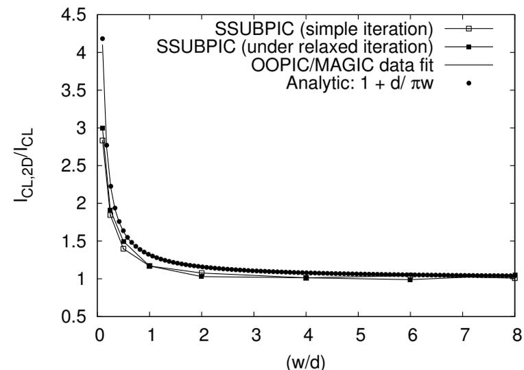
Under-relaxed iteration refers to averaging fields from two prior sets of simulation particles.
