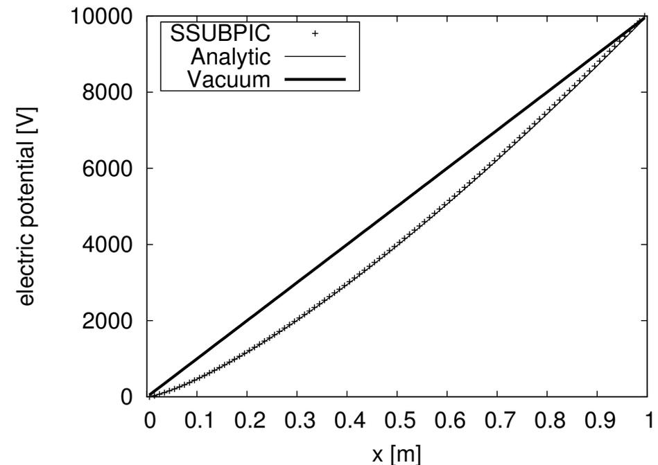
Potential profile for 100 cells in  $x$ -direction. Electrons originate from cathode at left and fly to the right. In the space-charge limited case  $E$  and hence  $dV/dx$  approach zero at the cathode to prevent further electron inflow.
