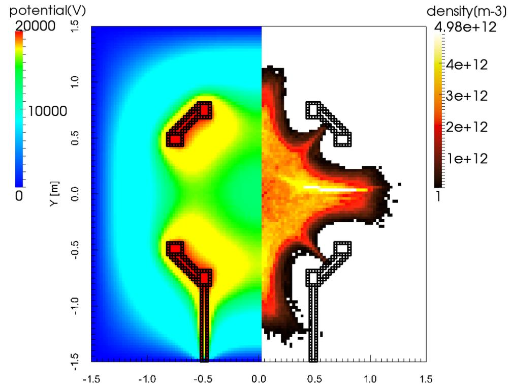
Electron number density and electric potential in converged solution.
