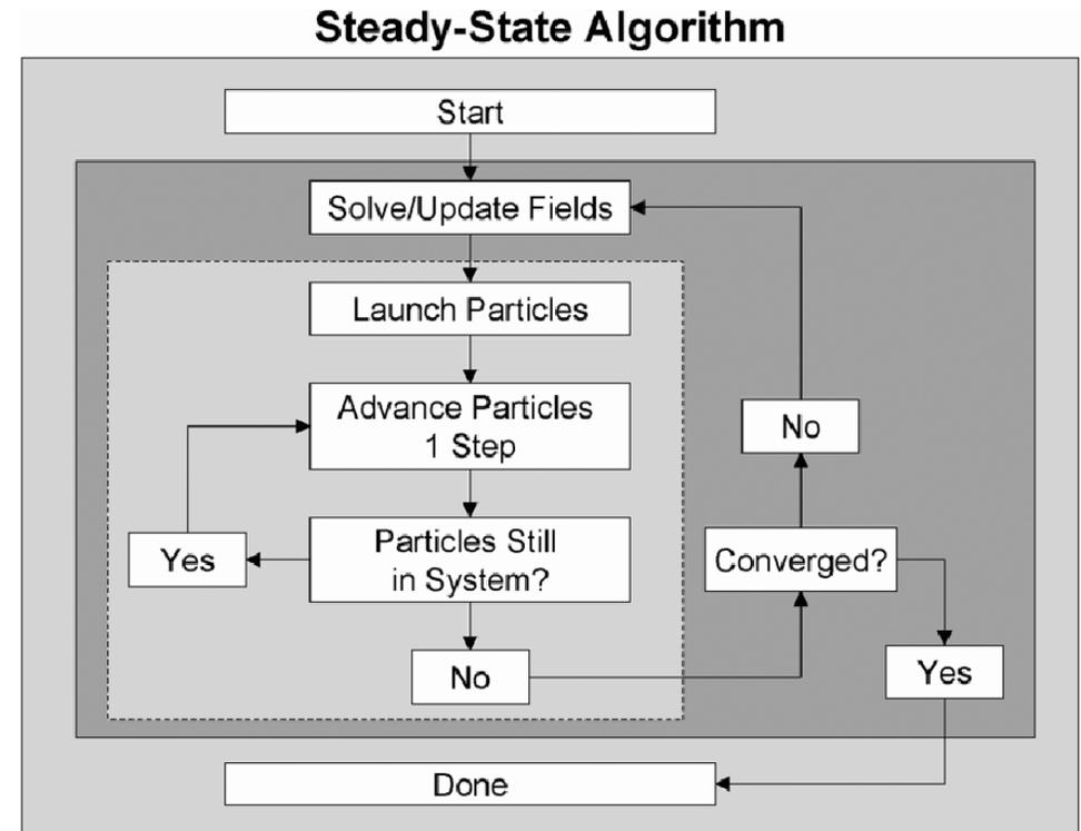
Scheme used by SSUBPIC and prior codes like MICHELLE. This image is taken from a Petillo et al [PND<sup>+</sup>05].
