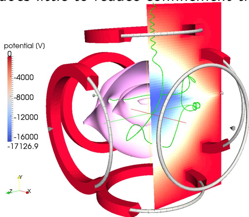
(a) Example orbit and potential contours. Coils (10 cm square cross-section) are grounded for field solutions.
