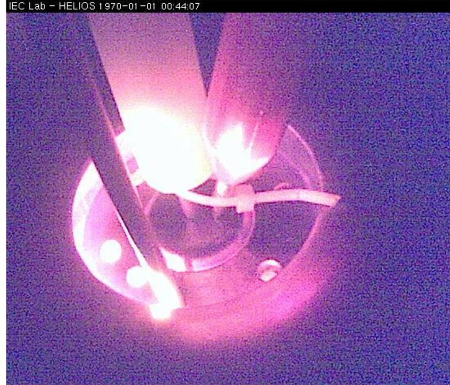
Initial Testing Failure: Internal Arc (corrected later)
